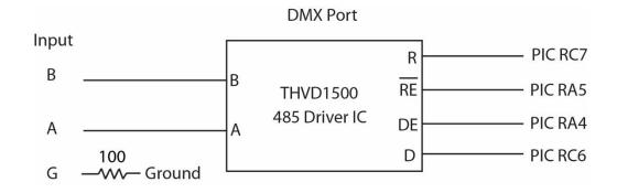
The DMX port is not isolated. Minimal transient suppression is provided internally by the THVD1500. This type of DMX receiver circuit will work fine for most applications. However some installations with mixed equipment and / or long wire runs may generate voltages that may damage the Hydra.
