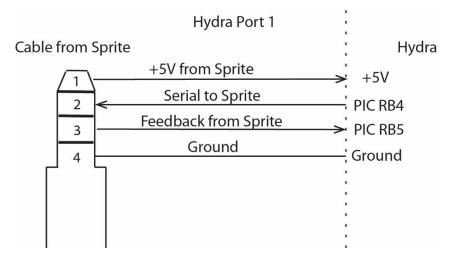
The Sprite media player connects to Port 1 of the Hydra. The Sprite will supply the 5 Volt power to the Hydra. The serial communications TX and RX are direct to the PIC processor on this port.
