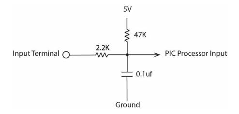
The Hydra input terminals 0 through 9 have a 2.2K series resistor to help limit current flow to a safe level for the PIC processor. There is a 47K pull-up resistor to bias the inputs to a High state. There is a 0.1uf capacitor to help reduce stray noise. For longer input wiring in electrically noisy environments, consider using shielded cable and / or adding capacitors to inputs.
