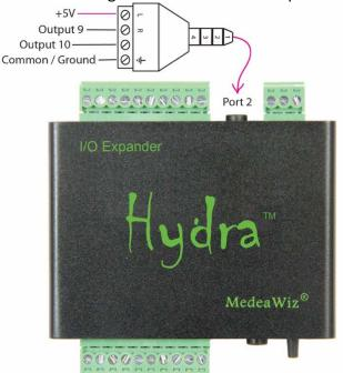
Outputs 9 and 10 connect directly to the PIC processor through a 180 Ohm resistor. For this reason the <u>safe output current is limited to 25ma</u>. A small indicator LED may be wired direct to these outputs. Outputs 9 and 10 are active Low and supply Ground to the external load device. For larger loads please use a SSR, or TTL logic level, or optical coupled type relay. Note we have found some relays are not isolated as advertised and may not work properly.
