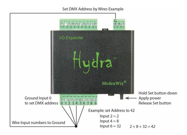
Input 0 must be grounded to let the Hydra know you want to set the DMX address . Values of any Inputs 1-9 that are grounded will add together to make the address.
