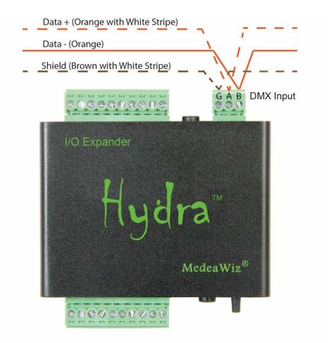
The DMX Port should only be connected to a DMX 485 bus device. Standard A, B and Ground / Shield terminals are provided. Commonly used colors are shown for Cat 5 cable above. Your colors may vary. DMX wiring for XLR and RJ45 connectors are shown below.
